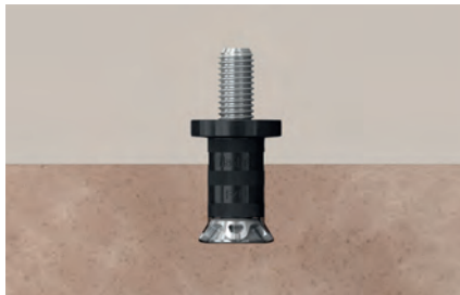
Stand-off installation in natural stone
